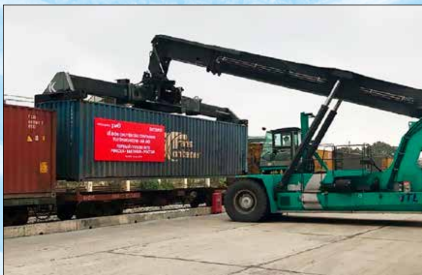
Loading of a container on a flat wagon for delivering in direct railway service between Russia and Vietnam
