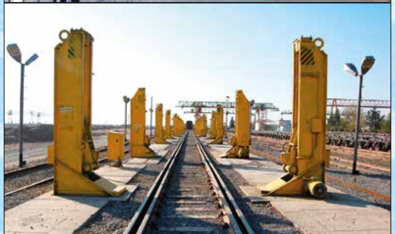
Boggie-changing points: top – at Byelorussian-Polish border, below – at Turkmenistanian-Iranian border
