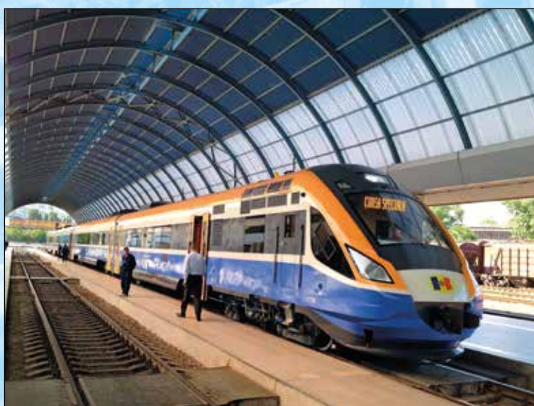
Diesel multiple unit D1 modernized by the company Remar Pascani (Romania) for CFM (Moldova)
