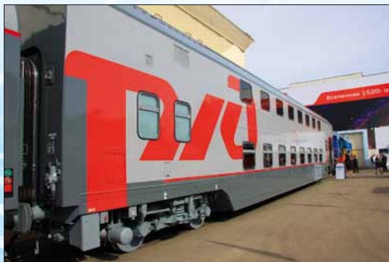
A new experimental double-decker sleeping car of RZD JSC
