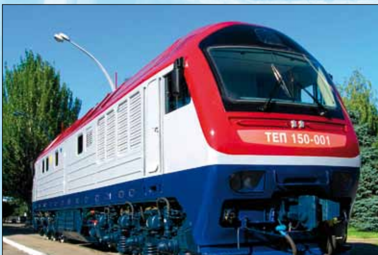
TEP 150 – a long-distance six-axle passenger diesel locomotive with electrical transmission manufactured by the Lugansk Locomotive-Building Plant on the Ukrainian Railways
