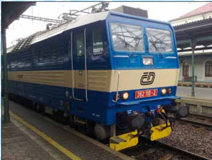
A modernized electrical locomotive of CD (Czech Railways)
