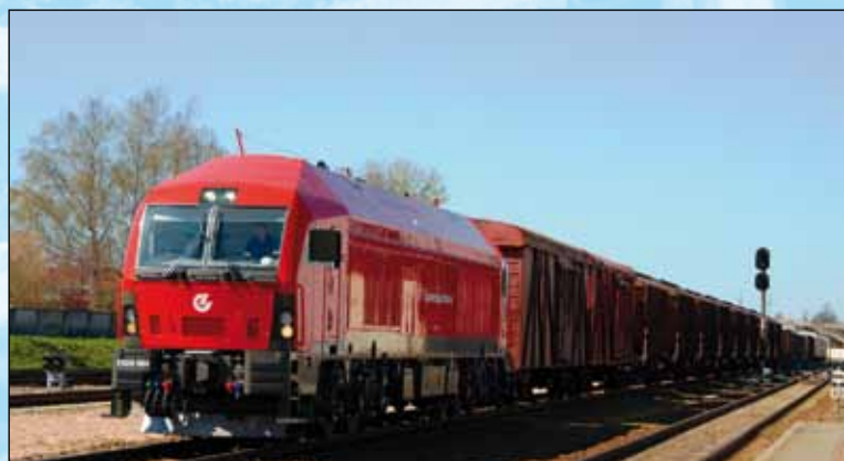
A new freight locomotive ER20CF of LG (Lithuanian Railways) manufactured by Siemens
