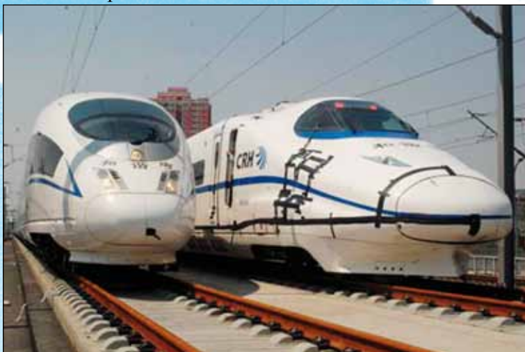
CRH-series high-speed train of Chinese Railways for movement of up to 350 km/h at high-speed railway line Peking (Beijing) – Tianjin
