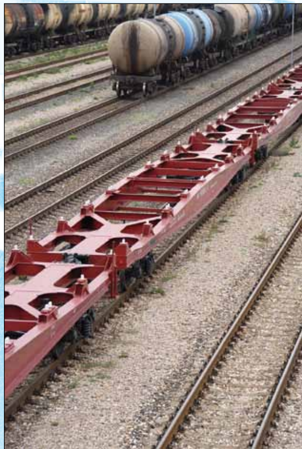
New 1520-mm open platforms for domestic and cross-border traffic between OSJD countries (Latvian Railway)
