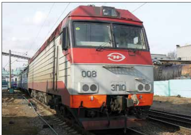
EP10 two-system passenger electrical locomotive, manufactured in Russia together with Bombardier
