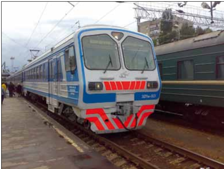
ED9MK Express enhanced-comfort emu arriving from Volgograd at Saratov station (RZD, Russia)
