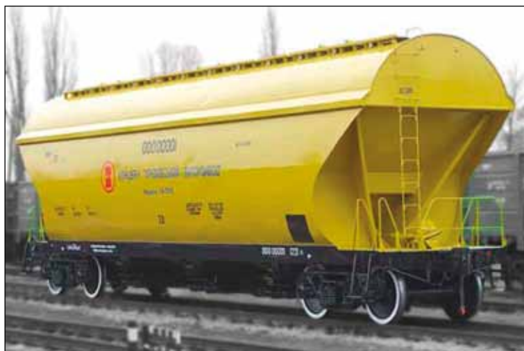
A modular hopper car 19-7016 series for transportation of grain crops and other bulky goods, which require protection against precipitations, on 1520-mm tracks (UZ, Ukraine)
