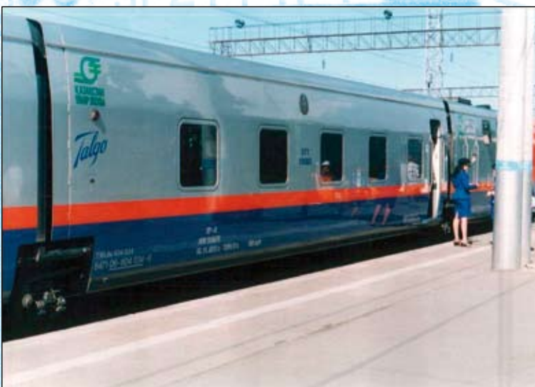
The sleeping-car of the Spanish train "Talgo 200", contains 20 sleeping berths or armchairs in 5 compartments. Alma-Ata 2 station, Kazakhstan
