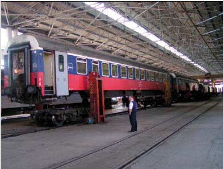
Train trip Wien - Moskva: Inside regauging hall at Brest - sleeping car Wien - Moskva
