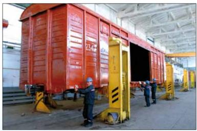
Overhaul repair of rolling stock for UTI (Uzbekistan)
