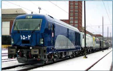
The Euro-Sprinter ER 24 manufactured by Siemens for RAI (Iran) (photo: A. Dworaczek)
