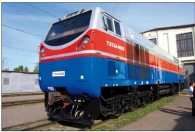
Diesel locomotive TE33A (Evolution) manufactured in Kazakhstan
